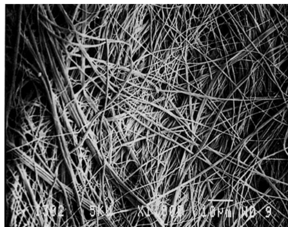
Figure 7 SEM photomicrograph of polypropylene microfibers produced via extraction of PVOH/PP blend (see Fig. 6).
